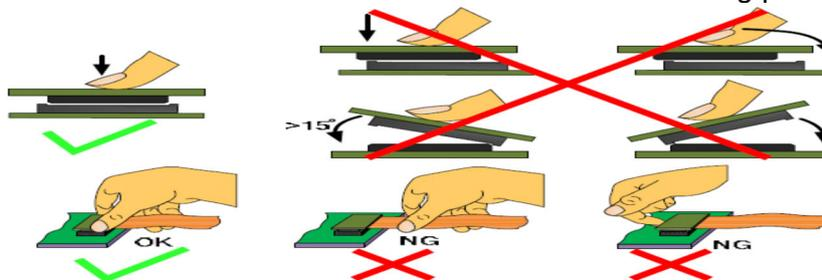
**5. Precaution for soldering the LCM**
